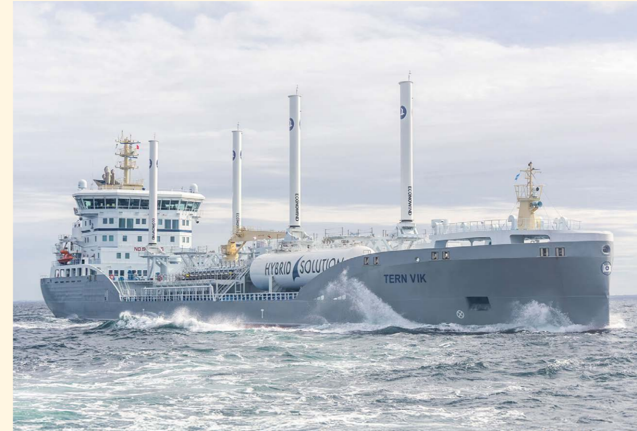
Terntank's latest tanker has retractable sails for wind-assisted propulsion.
